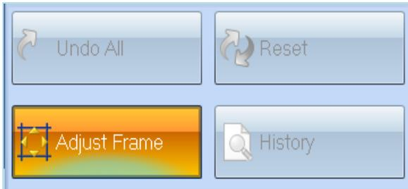
→ Select 'Adjust Frame'. Drag the graticule out to include the area you want to count colonies in. The software will not perform an automatic count of the area. Press 'Adjust Frame' again to complete this step
