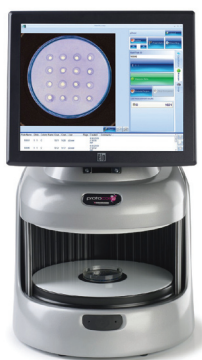
The ProtoCOL 2 from Synbiosis measures zones of inhibition during antibiotic and vaccine testing.
