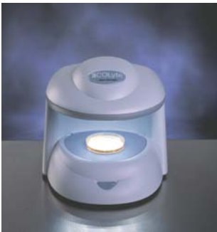
Figure 1: An aCOLyte SuperCount colony counting system
