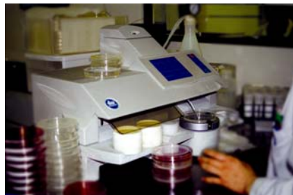
Figure 1: The WASP spiral plater used at I & A Lab for plating out milk samples.
