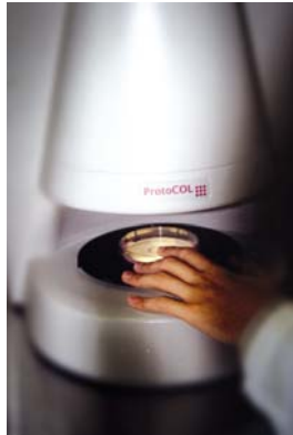
Figure 2: Synbiosis ProtoCOL system used at I & A Lab for automating counts of small colonies sampled from milk.
